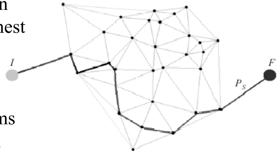
Figure 5 - Sensor Field With Weighted Delaunay Triangulation And Maximal Support Path ( P_s )
